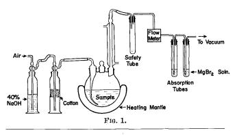
*Procedure.* Place 400 g. of sample in a 3-liter flask and attach to the apparatus assembly. Pipette 20 ml. of magnesium bromide solution (500 g. in one liter of 0.02 N sulfuric acid) into each absorption tube. Draw air at the rate of 1 to 1.5 liters per minute through the equipment for a period of one hour. This aeration is performed without heating.
